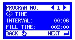
Here you can set a parameter. The top line shows which value is to be set. The next line indicates the possible range of values. An entry is possible directly by means of the number keys or by selecting the digit with the right / left arrow keys and by setting them with the up / down arrow keys. The selected digit is displayed inversely (cursor). Confirm the entry by pressing the ENT key or abort it by pressing the BACK key (in this case the initial value is not
